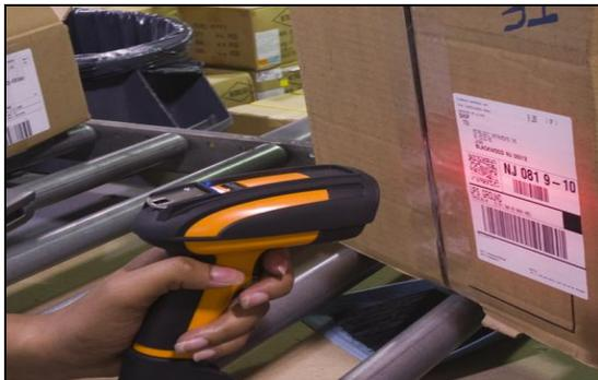
During all the In-Bound processes ( and at Stock Opening Balance) the system stores the scanned barcode info, along with the other storage specifications. During all the Out-Bound processes the system automatically fetches the storage info of the material on the scan. So, the system maintains absolute tracking of each and every piece of the material stored in the warehouse.
